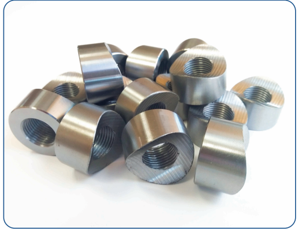
coding example: B22-R30 M18X1.5 OR M22X1.5 RADIATED PORTS FOR WELDING ON THE CYLINDER TUBE
