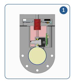
cesses and supplies the linear position of the cylinder rod. Section 2 shows the perfect axial and radial alignment of the bearing with the center of the rod, obtained with the insertion of two
