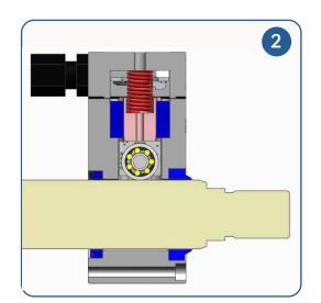
guide pins between the internal parts of the receptacle and the external ones of the fork inserted in it, to guarantee perfect detection of the angular movement of the transduction mechanism.
